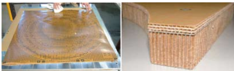
Copper patches on Kapton layer (left) integrated into Aramid-Carbon-sandwich (right)
