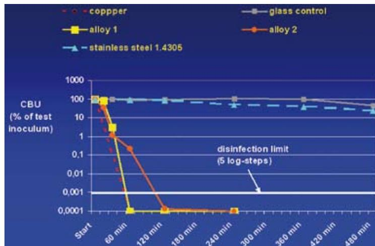
Fig 1: Results on the test JIS Z 2801 [8] with copper, Cu-alloys and stainless steel coupons. The inoculum (Staphylococcus aureus ATCC 6538) was about 1.000.000 cfu (colony forming units) per coupon (50 \* 50 mm) each. A reduction rate of > 5 log steps is needed for disinfection.
