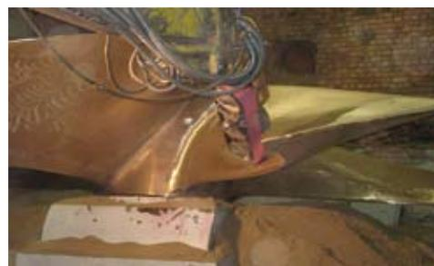
Fig. 1: Grinding of the propeller
