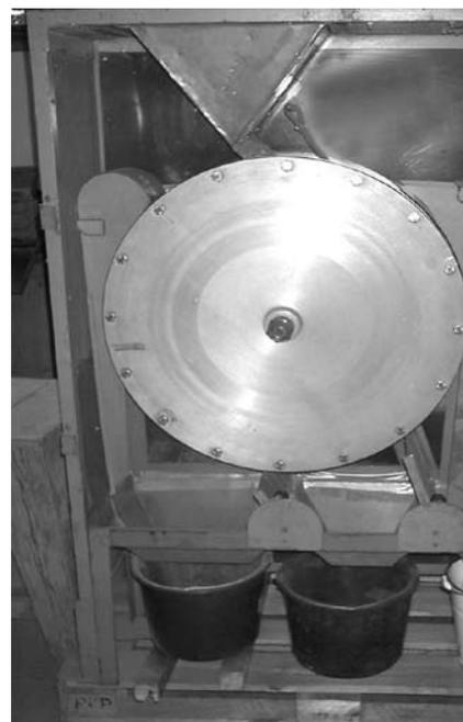
**Fig. 2: Rotating drum magnetic separator**
